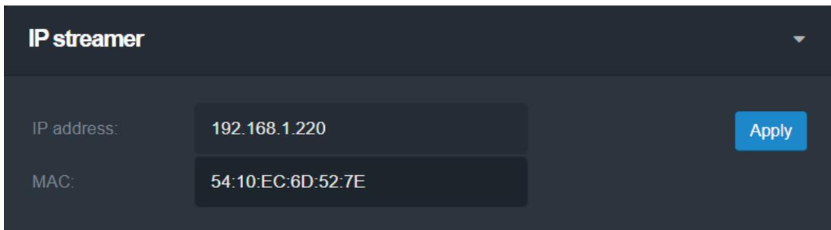
The IP streamer section provides the IP address of the headend's streamer that can be used for PING purposes as well as its MAC address.
