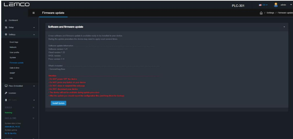
The device automatically downloads the available firmware update from the cloud server and notifies the user that there is a new firmware update. The user by clicking the “Install” button the device does the update automatically and reboots itself...
