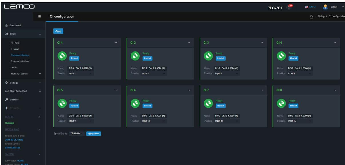
For each CI interface (CI1 to CI8) the user is able to select if the CI will be connected at the input or at the output using the "Position" field as follow:
