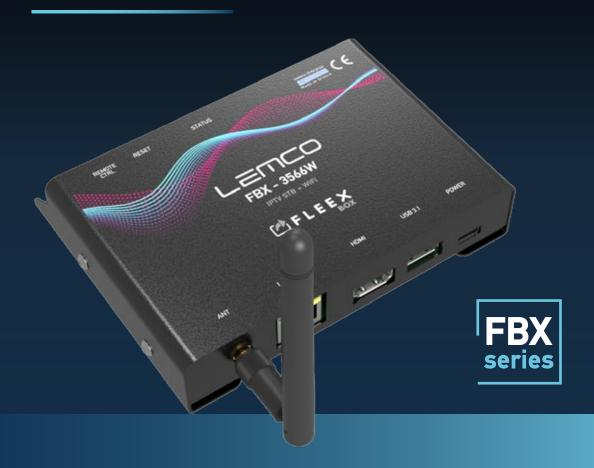
Boasting a high-performance quad-core A55 CPU clocked at 2GHz, coupled with 2GB DDR4 memory and a Mali-G52 GPU, this device is a powerhouse of efficiency and speed. Its specialized lightweight Linux OS ensures peak performance and ultra-fast booting.
