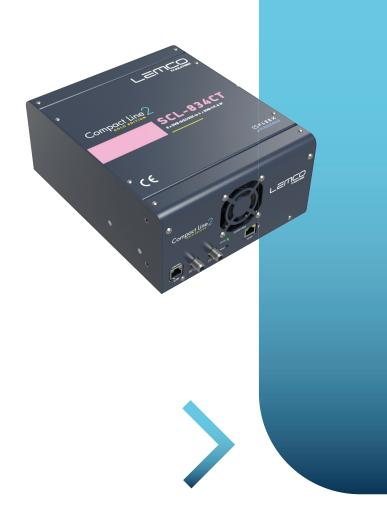
The SCL-834CT headend from Lemco's Compact Line 2 series is a highly versatile and efficient all-in-one device designed to accommodate diverse broadcasting needs. Its advanced capabilities include the ability to receive up to 8 independent signals from satellite (DVB-S/S2/S2X) with multi-stream support, converting them into 4 DVB-T/C RF output channels while simultaneously offering 1 Gbit IPTV streaming.
