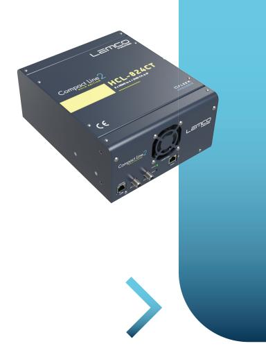
The HCL-824CT headend from Lemco's Compact Line 2 series is a state-of-the-art, all-in-one device designed to accommodate a wide range of broadcasting needs. With the ability to receive up to 8x HDMI signals, it efficiently converts them into 4 DVB-T/C RF output channels while simultaneously providing 1 Gbit IPTV streaming.
