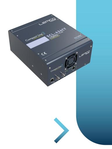
The SCL-434CT headend from Lemco's Compact Line 2 series is a highly versatile and efficient all-in-one device designed to accommodate diverse broadcasting needs. Its advanced capabilities include the ability to receive up to 4 independent signals from satellite (DVB-S/S2/S2X) with multi-stream support, converting them into 4 DVB-T/C RF output channels while simultaneously offering 1 Gbit IPTV streaming.
