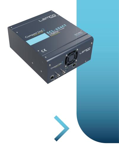
The SCL-424CT headend from Lemco's Compact Line 2 series is an advanced and powerful all-in-one device, designed to meet diverse broadcasting requirements. Capable of receiving up to 4 independent satellite (DVB-S/S2), terrestrial (DVB-T/T2), or cable (DVB-C) signals, it converts them into 4 DVB-T/C RF output channels while simultaneously providing 1 Gbit IPTV streaming.
